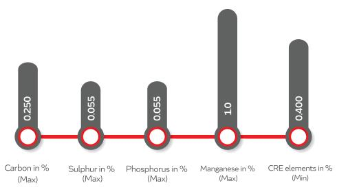
\*CRE - Corrosion Resistance elements like Copper, Nickel & Chromium
